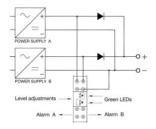
Monitoring two power supplies in redundant operation.
