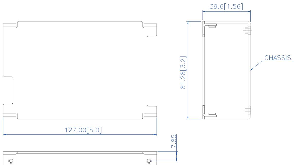
F Type (U-Chassis with built-in Top Fan): 5(L) x 3.2(W) x 2(H) inches; Weight: 500g (single output) / 550g (dual output)
