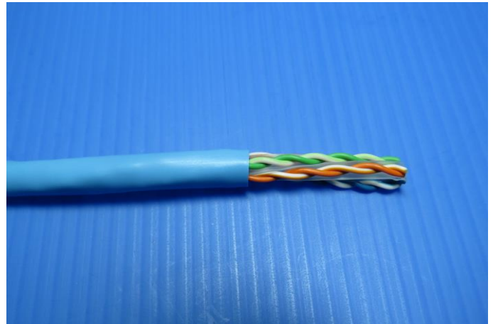
2. Strip cable jacket around 30mm.
