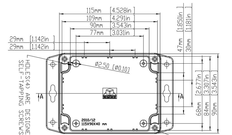
HOLES(4) ARE DESIGNED FOR SELF-TAPPING SCREWS USE.
