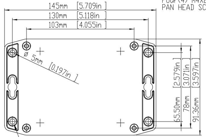
HOLES(4) ARE DESIGNED FOR M4 PAN HEAD MACHINE SCREWS USE.
