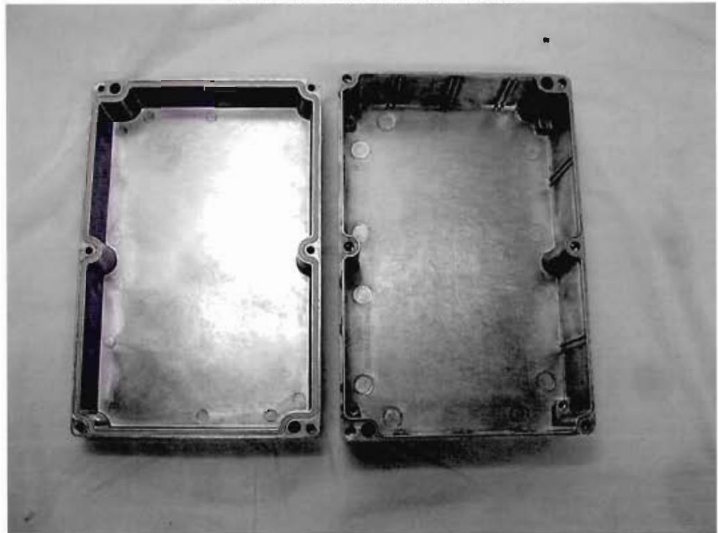
There is no trace of water inside.
