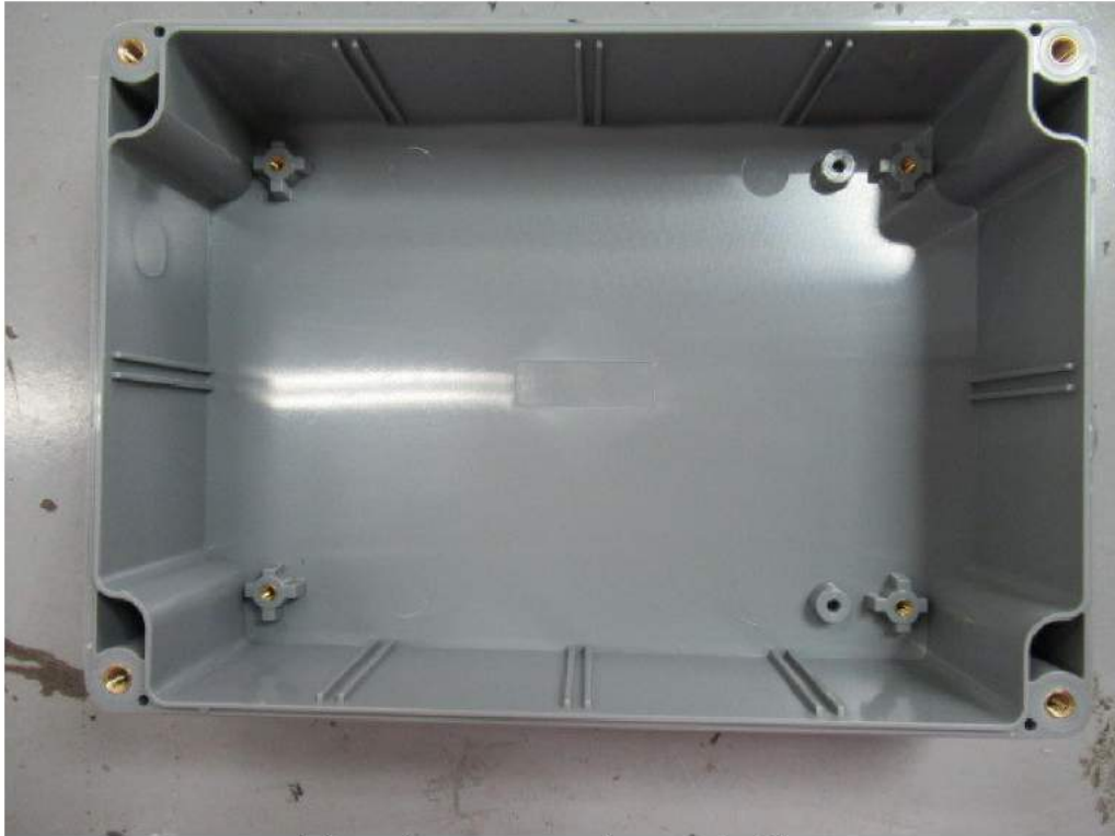
There is no trace of water inside.
