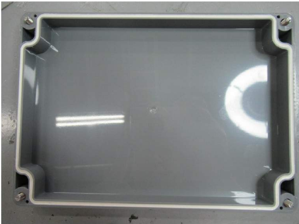
There is no trace of water inside.
