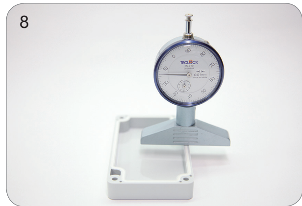
Check the depth and make sure the adhesive installation is OK
